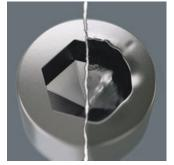
Hexagon screws can endure a problem because the contact surfaces delivering the power from conventional the tool, transferred to the screw via very small surface areas. The consequence: the screw can become damaged (rounding out). Hex-Plus tools have a greater contact surface that prevents this from happening! At the same time, as much as 20 % more torque can be applied. Good to know: Hex-Plus tools fit into every standard hexagon socket screw!
