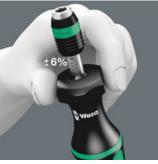
Simple setting of the required torque by hand. Easy-to-read scale value. Measurement accuracy is ± 6 % in accordance with the standard EN ISO 6789. Distinctly audible and noticeable excess-load signal when the pre-set torque is reached.
