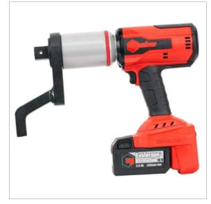
The EvoTorque® Battery Tool (EBT) features a new brushless motor, data memory and data transfer capabilities. Norbar have combined this with their respected gearboxes to deliver a range of fast, reliable, accurate battery torque tools **Part number**: 180445 **EAN Bar Code**: 5060922230157 **NATO number**: -**Accuracy**: Up to ±3% **Operates between**: 200.00 - 1350.00 N·m 150.00 - 1000.00 lbf·ft
